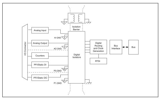
Figure 2-2. General NI 6232/6233 Block Diagram
